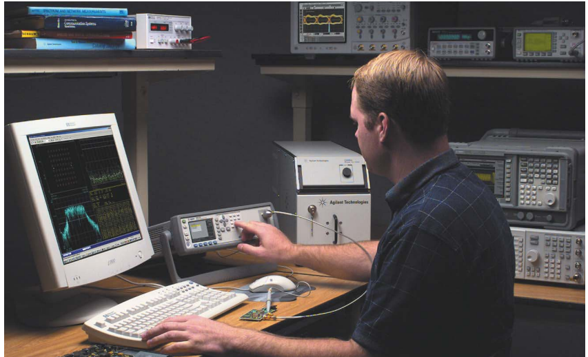
Testing a WiFi design requires a combination of RF- and data-level test equipment that designers must use together to fully exercise the protocols (courtesy Agilent Technologies).
