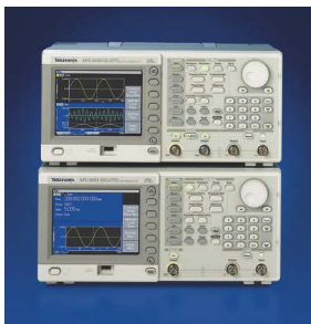
The AFG3252 (top) and the AFG3251 (bottom), two- and one-channel arbitrary function generators, reconstruct waveforms at rates as high as 2G samples/sec.
